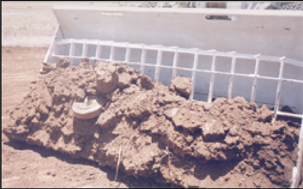
Figure 5G-3: Front-loader bucket with gill
