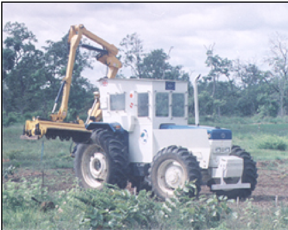
Figure 5G-4: Vegetation cutter on armoured tractor
